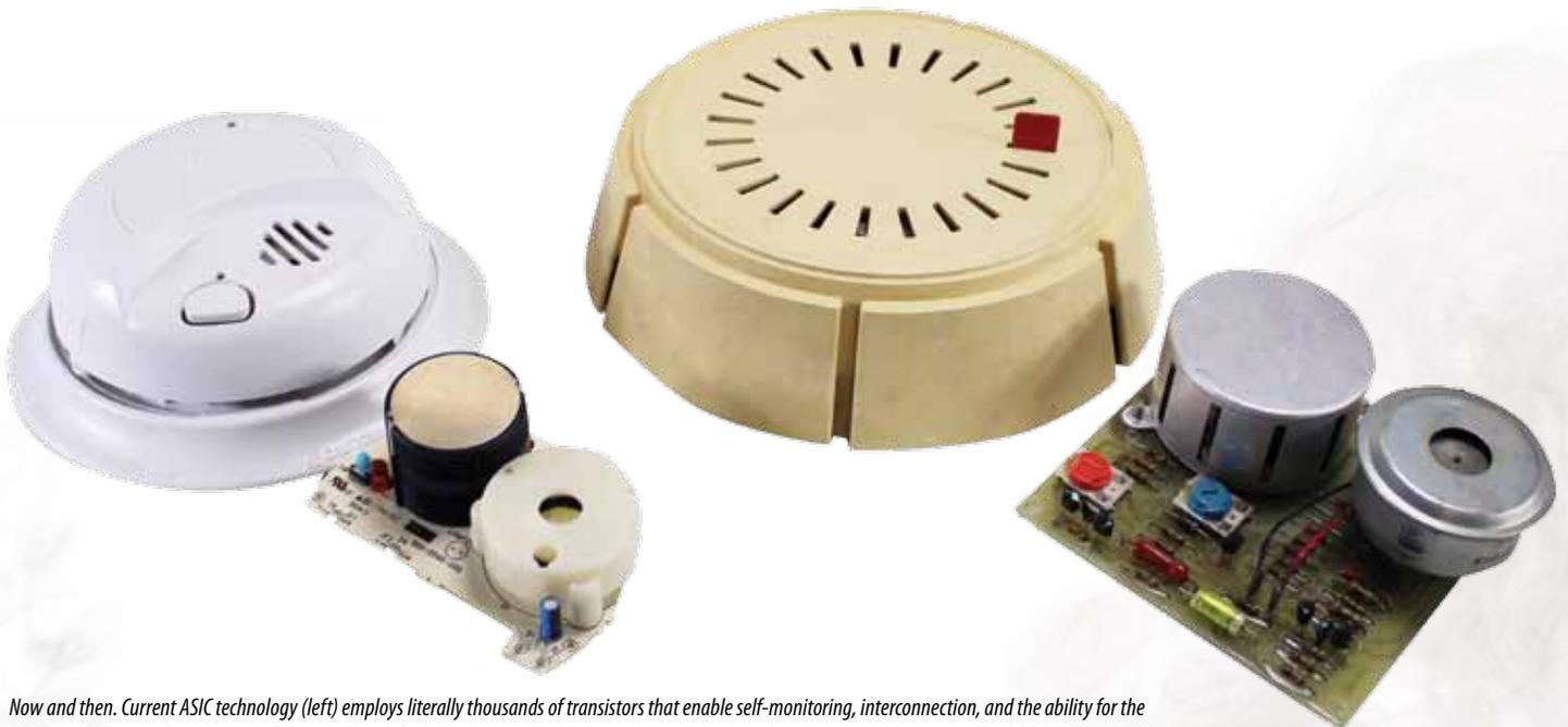
*Now and then. Current ASIC technology (left) employs literally thousands of transistors that enable self-monitoring, interconnection, and the ability for the battery to last more than a year. Early smoke alarms (right) had about one hundred components and a few transistors. Photo courtesy of Jarden Safety*
